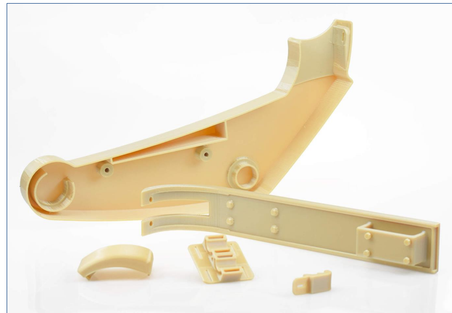
(Above) Brackets 3D printed on the Fortus 900mc Production 3D Printer. (Photo: Stratasyss)
